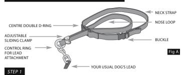
Attach lead to Control Ring (Fig A).
